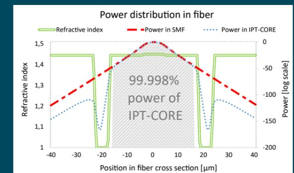
Fig. 6. Refractive index distribution in a MCF (green) and power distributions of the fundamental mode of a MCF (blue) and of a single-mode (red).
